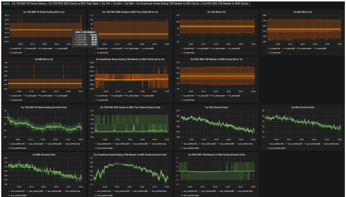
Figure 3.12: The *Grafana*-based long term logging web interface showing 1 h worth of data recorded for some of the locks in the  $^{40}\text{Ca}^+$  laser system. The orange plots in the top half show the error signal input streams, the green plots in the bottom half the corresponding PI controller output. In the latter, slow drifts in the laser controllers and/or reference cavities are apparent.
