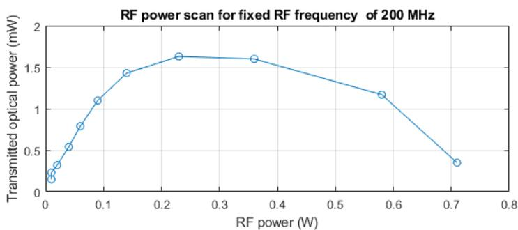
Figure 5: Transmitted optical power from the AOM as a function of the RF power coming from the RF source and amplified by the amplifier. The frequency was set to 200 MHz which leads to a maximum transmitted optical power as shown in Figure 4. The power of the beam before the AOM was also  $P_{\text{beam}} = 28.5$  mW.
