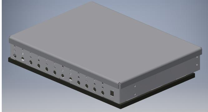
Figure 7: Aluminium box with removable roof on top of the water cooling plate. The water input and output channel of the cooling plate is at the back. The front panel is designed for maximal 12 amplifiers (12x2 holes for SMA, 12 holes for BNC and one hole for ethernet adapter).
