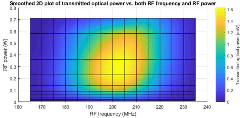
Figure 6: Smoothed plot of transmitted optical power from the AOM as a function of RF frequency and RF power.
