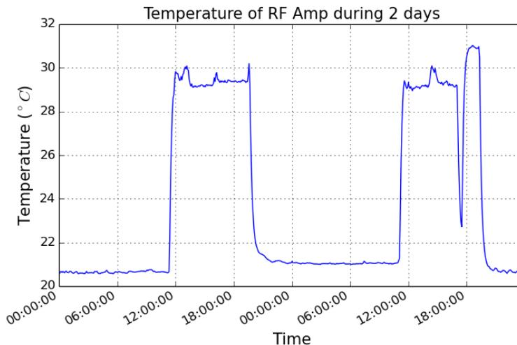
Figure 1: Temperature of *ZHL-1-2W-S(+)* RF amplifier during two working days. The temperature peaks correspond to daytime, where the amplifiers are being used.
