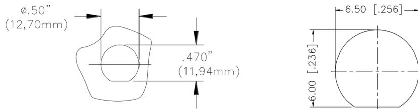
(a) Dimensions of the panel cut out for the BNC adapter
