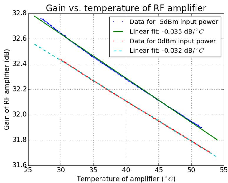
Figure 2: Gain of the *ZHL-1-2W-S(+)* amplifier measured as a function of the temperature for two different power inputs (coming from the TPI RF source): once with -5 dBm (top curve) and once with 0 dBm (bottom curve).
