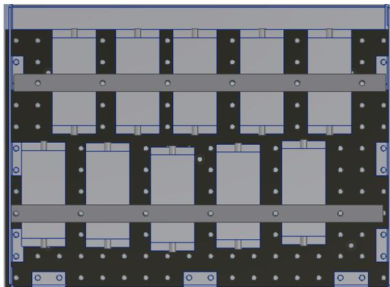
Figure 8: Top view of cooling plate with aluminium box but without roof. This is a possible arrangement for 10 amplifiers.
