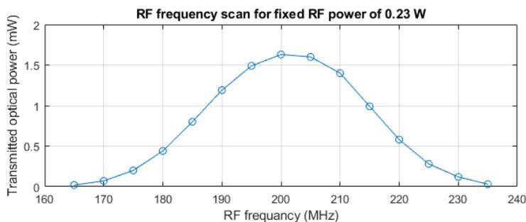
Figure 4: Transmitted optical power from the AOM as a function of the frequency of the RF source. The RF power was set to 230 mW which produces the maximal transmitted power, as shown in Figure 5. The power of the beam before the AOM was  $P_{\text{beam}} = 28.5$  mW.
