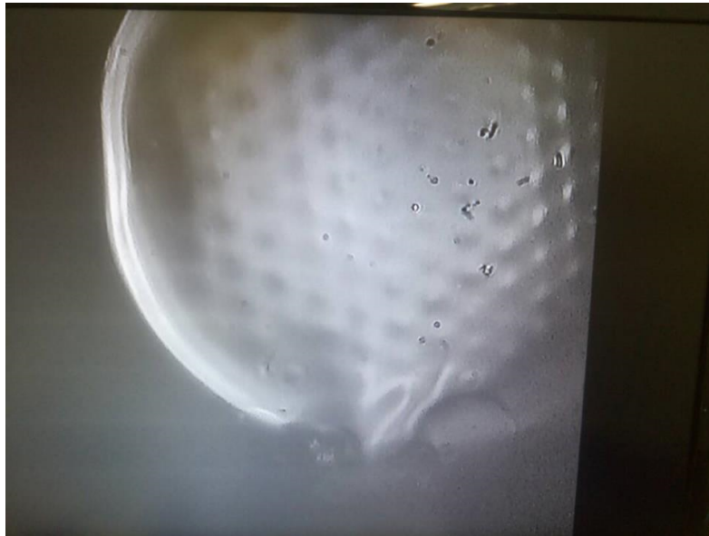
Figure 2.4: Collapsed tip surface of LMA-25 using our novel collapsing method.
