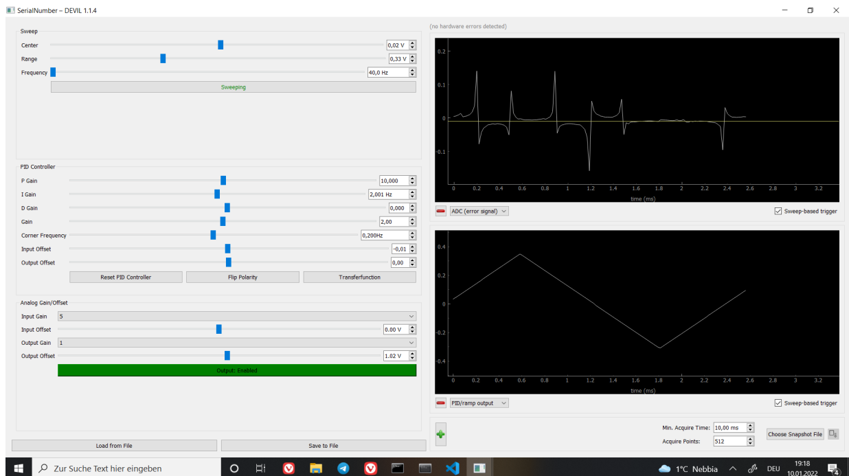
Figure 13: Picture of the GUI displaying a PDH signal. The structure has been kept the same, the only thing that changed visually is the left side with the sliders.
