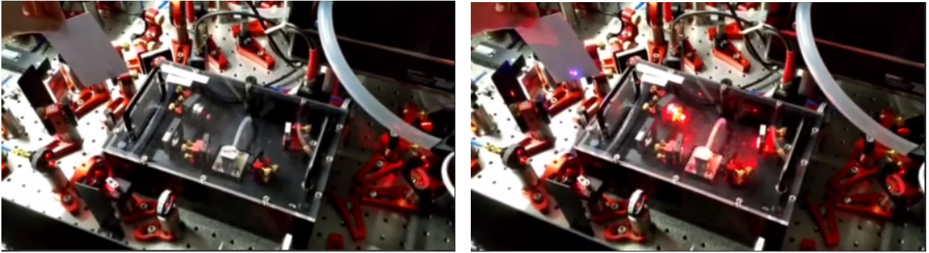
Figure 19: Screenshots of a video showing the locking process. While on the left the cavity is not on resonance with the laser, on the right the cavity freq. has been locked to the laser. The laser is now resonant in the cavity, which can be seen from the red radiation being scattered by the air, and the violet spot on the paper indicating that UV light is being emitted.
