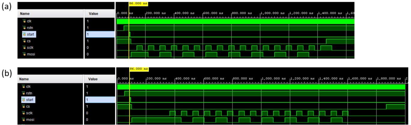
Figure 22: Comparison of the changes made to spi_master.v . (a) The behavior of the original version of the module. (b) Adapted version needed to make it work with the AD5293. In both cases, the data sent is 0b1010_1010_1010_1010 .
