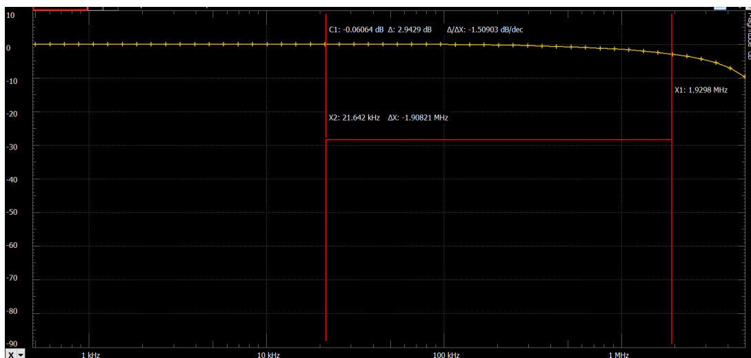
Figure 15: Measurement of the bandwidth of the input section 1 with G = 1 , measured for a signal of amplitude of 1V, taken with the Analog Discovery 2. The bandwidth was measured as the frequency at which the amplitude of the signal decreases of \Delta = 3 dB from its maximum. Here it is equal to 1.93 \pm 0.1 MHz.
