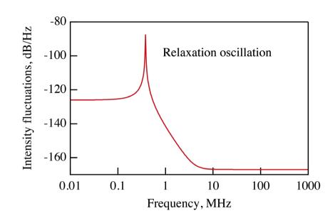
Relaxation oscillations in the time domain and frequency domain (microwave spectrum analyzer - not optical frequencies!)
