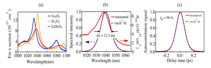
Given the quality of the available disks from the first growth run of Yb:ScYLO, we focused on exploring the limits in terms of pulse duration of this material, and were able to obtain 4.6 W of average power pulse duration of 101 fs. This was obtained at a repetition rate of 70 MHz, resulting in a pulse energy of  $0.1~\mu J$ . This result further confirms the potential of this family of materials for modelocking in the thin-disk configuration with short pulse durations.
