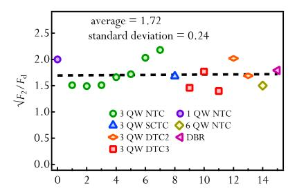
The data seems to confirm that the main contribution to IA and damage originates in the field in the DBR and spacer layers and not by the absorber section itself. This gives a clear indication of the damage behavior of such SESAMs, suggesting that catastrophic damage occurs due to heating of the lattice by energy absorbed by the IA process. It also indicates how to shift the damage fluence to higher values by simply increasing  $F_2$ .
