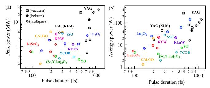
**Table 5.** Summary of results obtained with modelocked TDLs to date. Unless otherwise indicated, the oscillators were operated in air.
