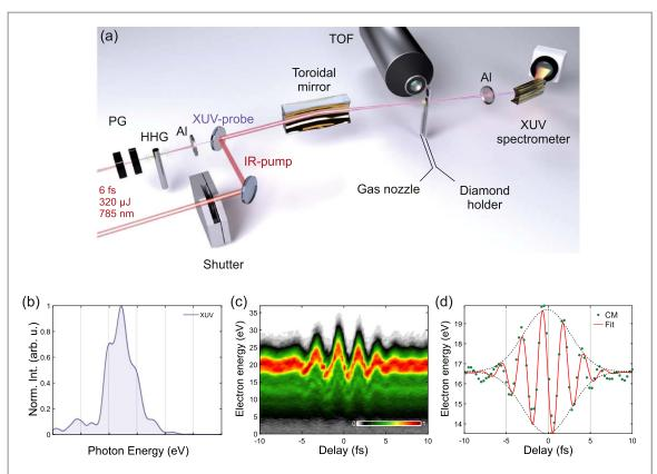
**Figure 2.** (a) Schematic of the experimental setup used for ATAS. (b) Attosecond pulse spectrum. (c) Streaking trace obtained in Ne with the pulse in (b). (d) Delay dependence of the photoelectron center of mass (CM) extracted from the trace in (c) (green dots). The red solid line represents a fit function, which is used to extract the negative IR vector potential:  $-A_{IR}(t)$ .
