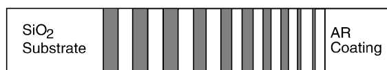
Fig. 3. Schematic picture of the universal structure of a double-chirped mirror. AR, antireflection.
