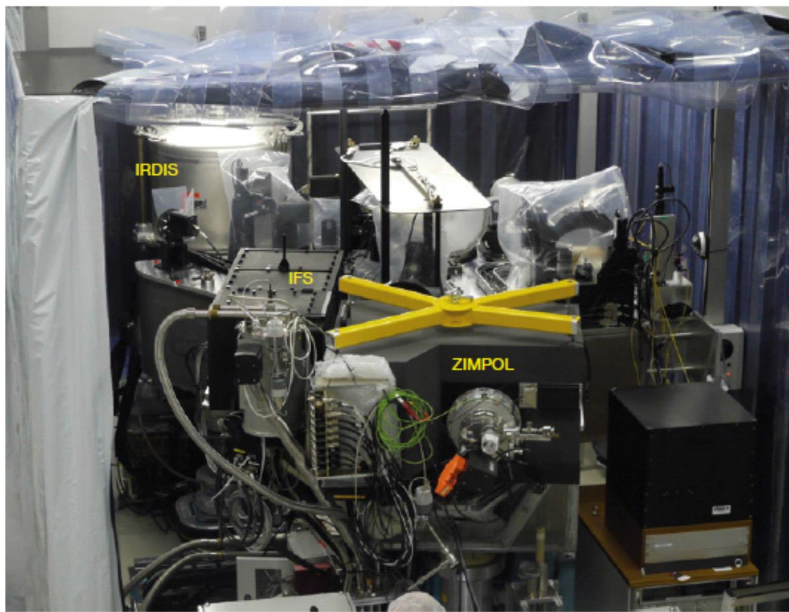
Figure 5. SPHERE in the assembly laboratory at IPAG with all instruments integrated into the common path.
