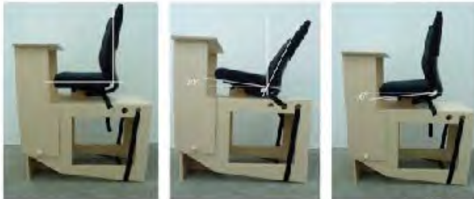
Figure 1: MRI-compatible chair in the three positions: upright (left), reclined (middle), and forward inclined (right).
