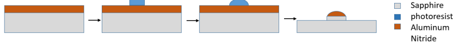
Figure 4.2.: Cross section of each part of the procedure for fabrication of the acoustic resonator.
