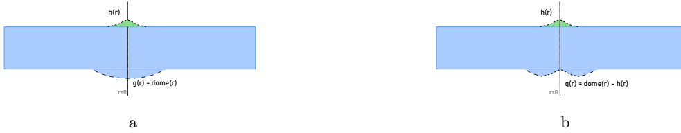
Figure 5.4: Two double-sided HBAR geometries. (a) The non-subtracted geometry and (b) the subtracted geometry. The subtracted geometry exploits an invariance of the acoustic Schrödinger equation, while the nonsubtracted geometry uses the approximately domical character of h . In both geometries, the piezoelectric is shaped according to the parameterised function h_A , but the opposing antipiezo structures are different. With the non-subtracted geometry, the antipiezo is simply a dome, whereas for the subtracted geometry it is a dome minus h . There are only three parameters for both structures, namely A \in [0, 2) , the height of the dome and its radius of curvature.
