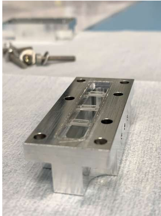
Figure 2.6: Open aluminium cavity containing three \hbar BAR devices from the w2274 wafer. The smaller HBAR chip is flip-chip bonded to the longer antennamon chip that rests on the cavity.
