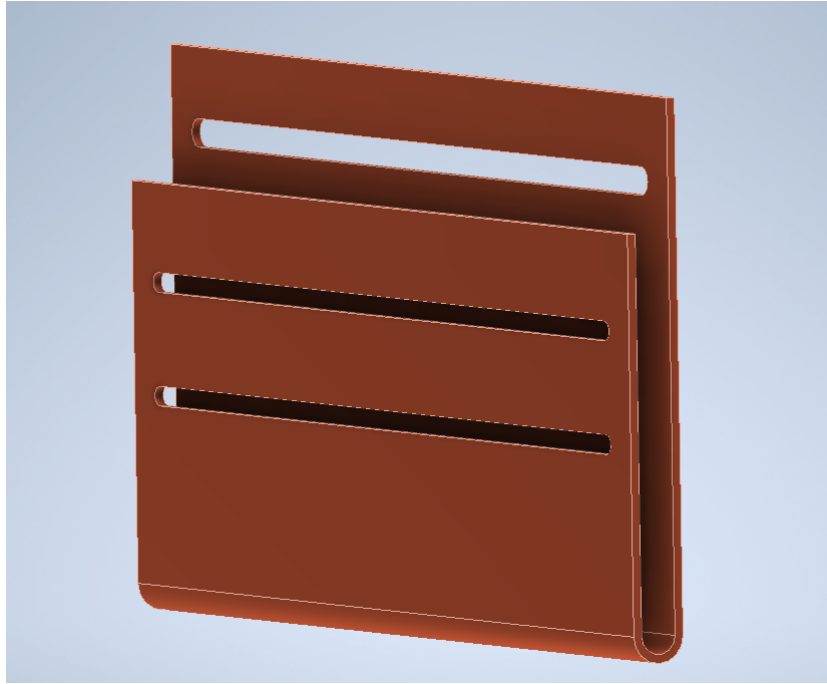
Figure A.2.: U-shape thermalizer. It is an example of a different thermalization solution compared to the one presented in subsection 3.2.1
