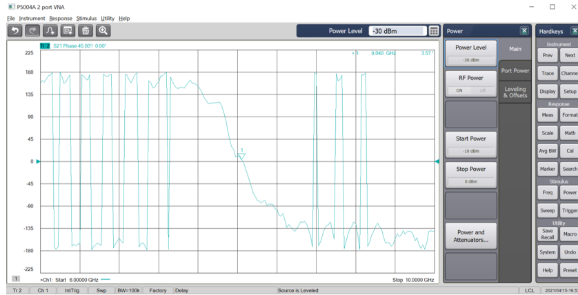
Figure 4.1: Screenshot of a VNA sweep. The resonant frequency of the SPA is at the point where there is no phase shift.
