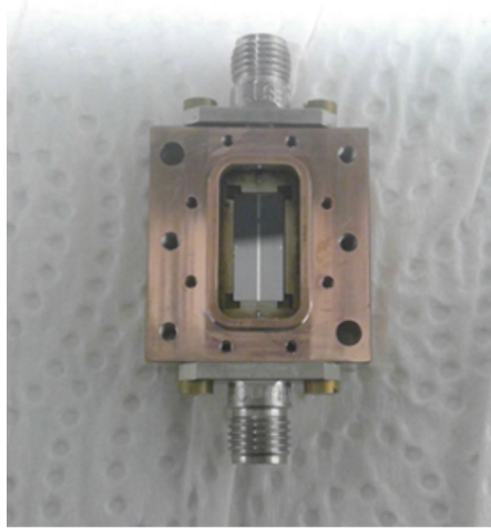
Figure 3.15: Assembled SPA without the lid and the magnetic field coil.
