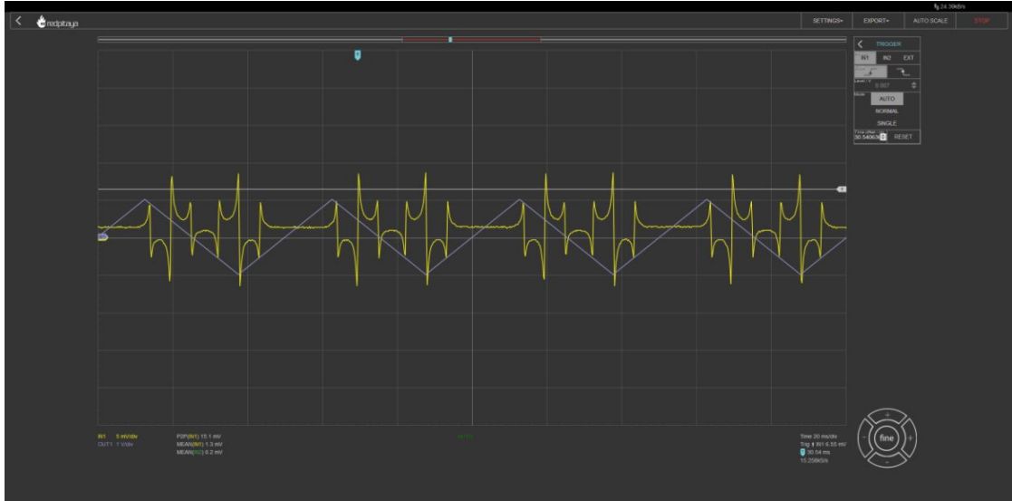
Figure 4.4: Experimental PDH error signal \epsilon .
