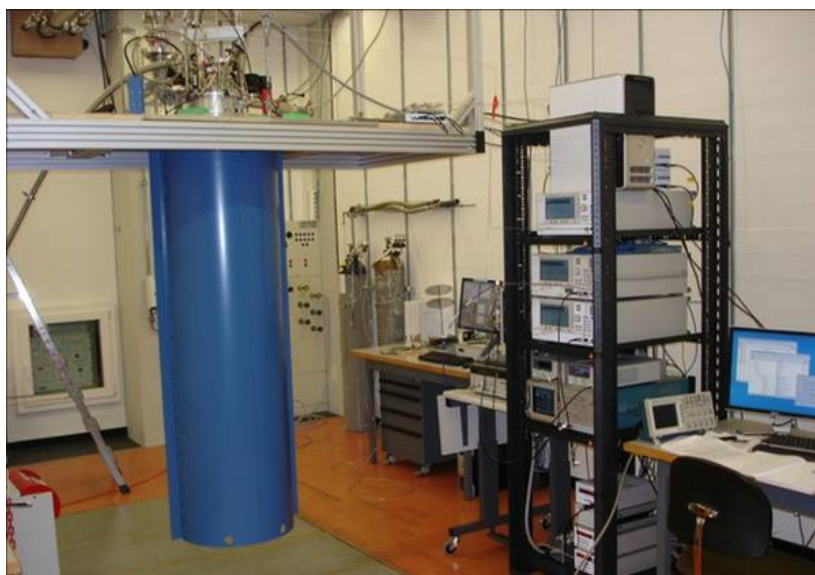
Figure 5.3: The experimental setup consisting of a dilution refrigerator wired for low noise and high frequency measurements and a rack of microwave electronic equipment including sources, up and down converters, digitizers and pulse generators.
