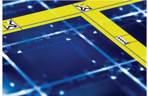
Figure 7.5: In our chip-based superconducting circuit three qubits are coupled to three resonators to realize deterministic quantum teleportation.
