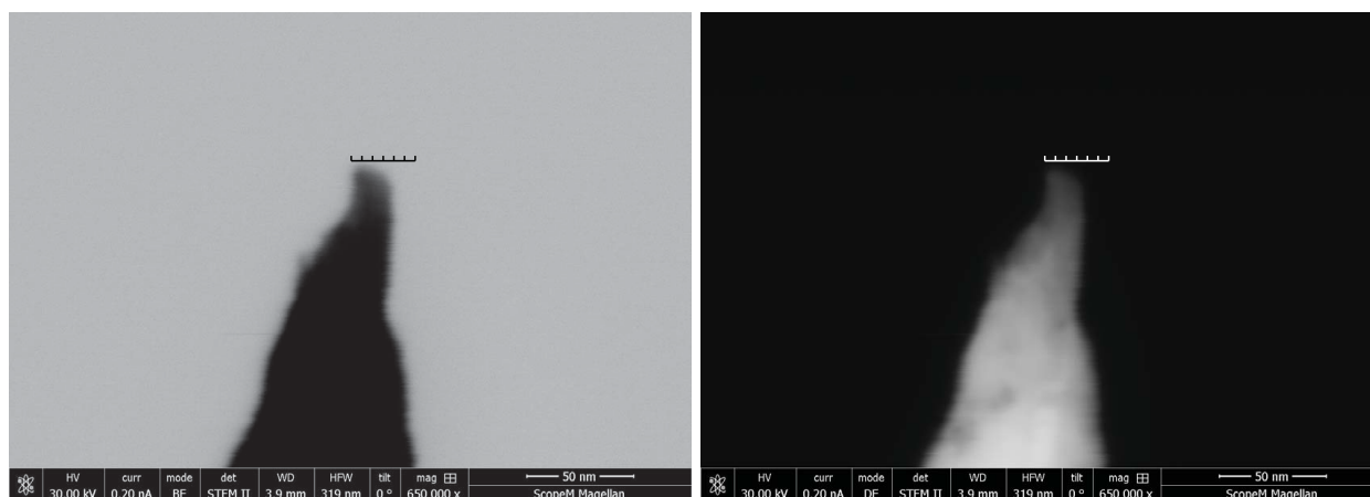
Supplementary Figure 3: Dimensions of tip B. Bright and dark field scanning electron micrographs of bare diamond nanowire tip. Ruler is 5 nm per tick. The estimated tip width is 18 nm.
