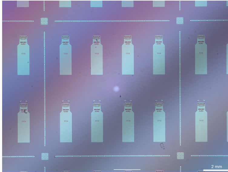
Figure S2: Wafer-scale fabrication of silicon nanoladders. Optical micrograph of chips carrying 6 nanoladders of different lengths after electron beam lithography and inductively-coupled plasma etching step. The chip dimensions can be easily changed during fabrication to allow mounting them in a variety of systems. Scale bar: 2 mm
