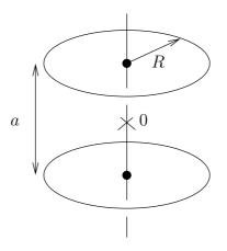
Let the two currents be equal, and oriented in the same direction. The set-up produces a magnetic field which is nearly constant within a certain area. More precisely: how should the distance a be chosen in order for  $B(x) - B(0) = O(|x|^4)$ ,  $(x \to 0)$ , to hold true?
