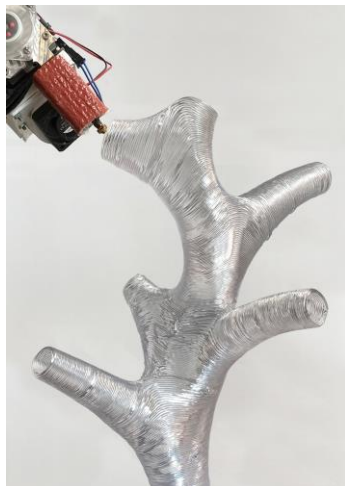
Non-planar FDM robotic 3D printing of branching structure. Photo credit: Ioanna Mitropoulou
