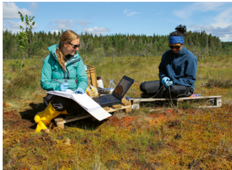
Push-pull test: Meret Aeppli and Prachi Joshi retrieve injected water from the bog soil and measure the remaining oxygen concentration.
