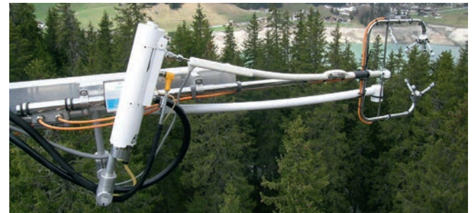
Current ICOS standard eddy covariance setup at Davos-Seehornwald, with a Gill HS-50 anemometer-thermometer and an enclosed-path LI-7200 IRGA.
