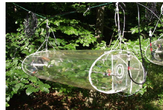
Set-up for measuring isotopic signatures of branch gas exchange
