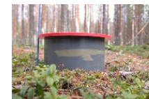
Soil respiration chamber
