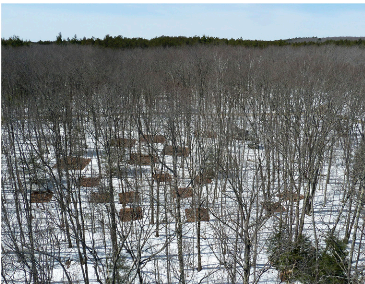
Researchers use these soil warming plots at the Harvard Forest Long-Term Ecological Research site in Petersham, MA, to study the response of soil biota to simulated climate warming. Plots have been warmed continuously to 5 °C above ambient temperatures for 10–24 years using buried heating cables. Control plots are still under snow cover. Image courtesy of Audrey Barker-Plotkin (Harvard Forest, Petersham, MA).
