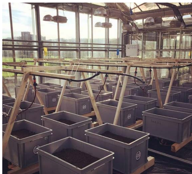
Figure 4 - In house built mesocosms for the greenhouse incubations
