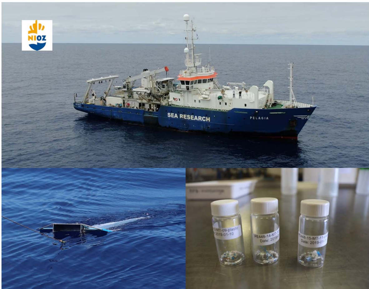
A manta trawl is used to collect microplastics. (Photos by Phillippe Delandmeter and Hans Limburg.)
