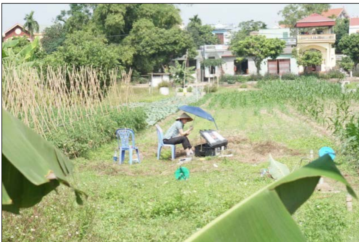
Fieldsite: Van Phuc, Vietnam; taking measurements of gases in groundwater using the miniRUEDI portable mass spectrometer.
