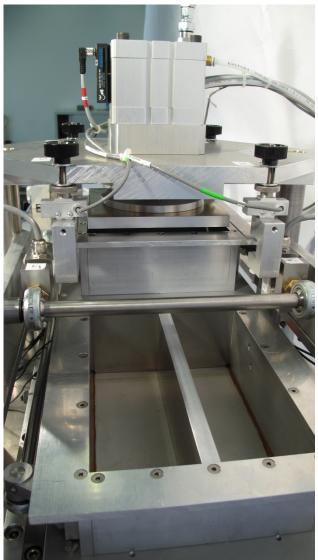
The lower frame is longer than the upper frame. Its bottom plate is a sintered stainless steel plate which is porous with an air entry value of approximately 200mbar (max. suction).
