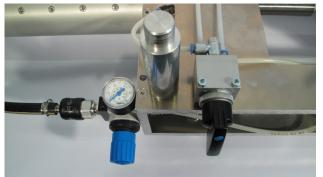
The consolidation stress is generated by air pressure and introduced with a pneumatic cylinder.
