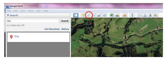
A new window ("New Polygon") opens. Mark four edges of a polygon that contains the region of interest (the polygon becomes white) and click "Ok".
