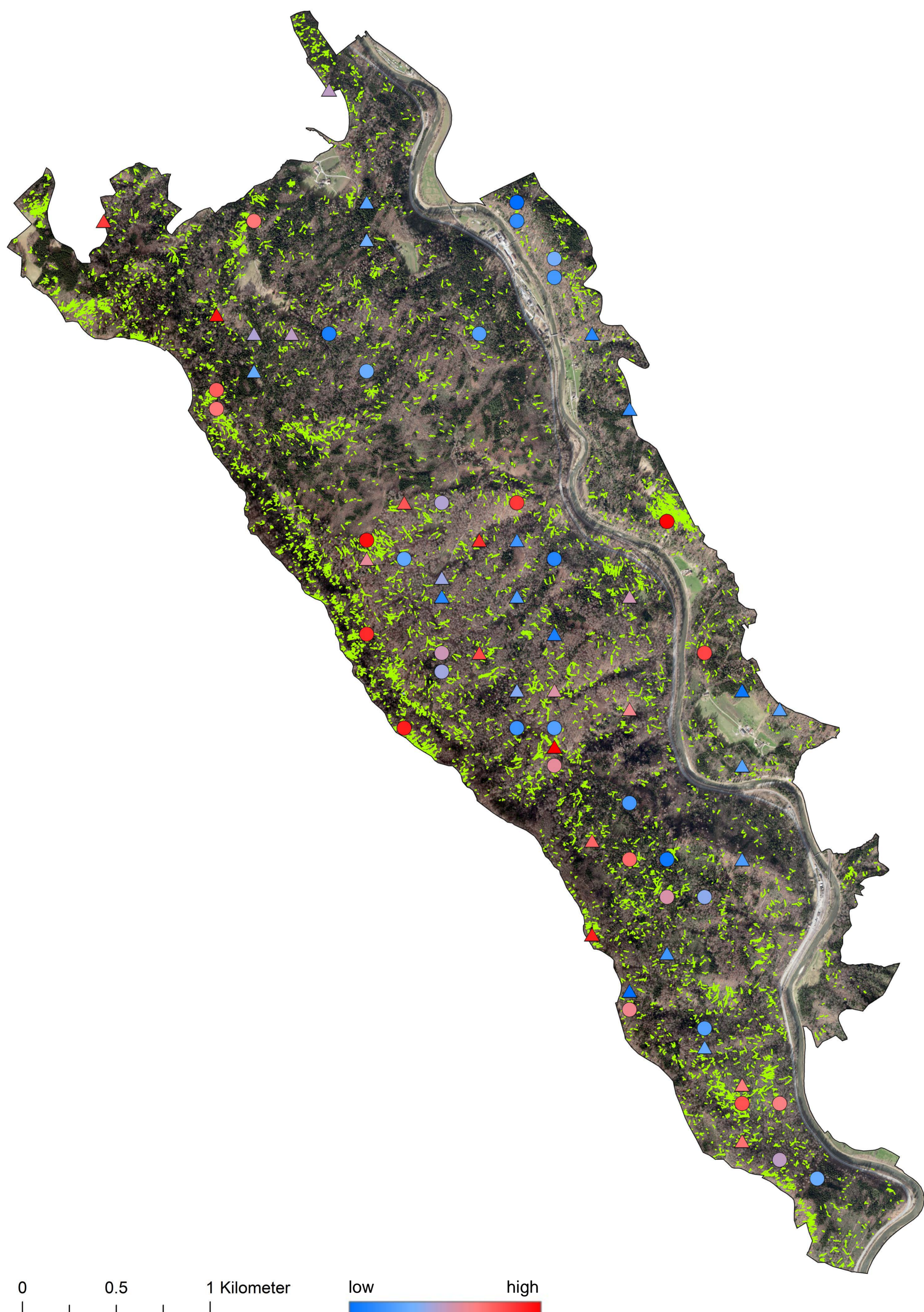
Figure 2: Deadwood-map of the Zurich Wilderness Park Sihlwald, created with LiDAR and 3D aerial photographs. 70 plots were chosen along two gradients: 1. deadwood amount (blue = low to red = high) and 2. connectivity (triangles = high and circles = low) (aerial photograph: 14.3.2014, Osterwalder, Lehmann – Ingenieure und Geometer AG).
