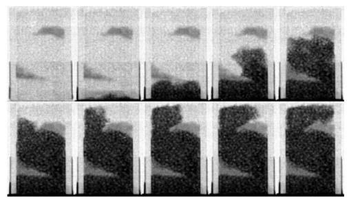
Time-series neutron radiography of an effect of microplastic (MP) (dark gray) on capillary rise of water (black) into sand columns (light gray). Water flows around MP in an elongated flow path increasing tortuosity and entrapping air around MP aggregations. (A. Cramer et al., 2021)
