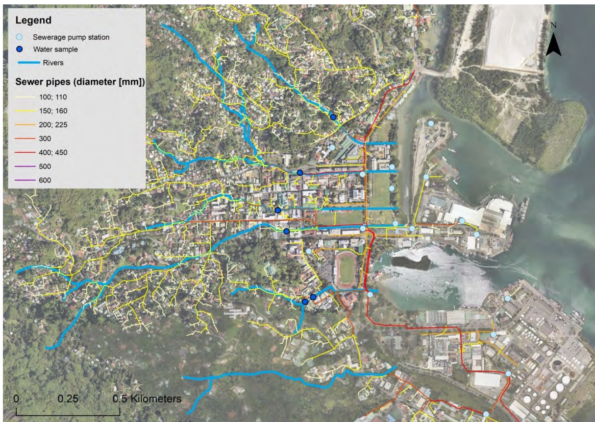
Figure 9: Sewerage network around Victoria (data provided by PUC, 2019 11 ).
