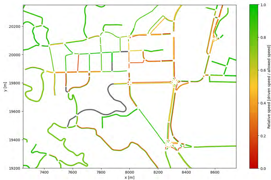
(b) Relative Speed in the GVA during the MPH, relative speed is defined as the driven speed on a single edge in relation to the allowed speed on this edge; modelled in the Mahé Simulation. The colour scale spans from red (low relative speed) to green (high relative speed). No values are available for the grey road sections because of restricted accessibility.
