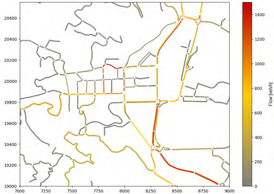
(a) Vehicle flows in the GVA during the MPH, modelled in the Mahé Simulation. The colour scale spans from grey (low traffic volume) to red (high traffic volume).
